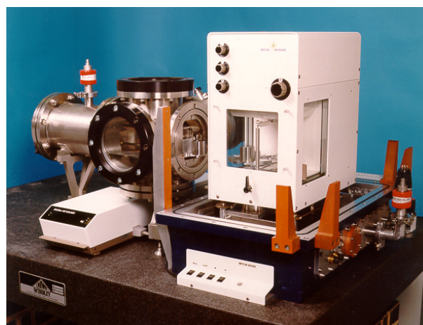
Fig. 1. Mettler HK1000MC mass comparator with base of vacuum chamber and load-lock mechanism.
