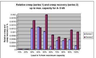
Figure 3: Relative creep and relative creep recovery in % versus load in % for A-5kN
