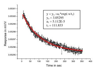
Figure 6: Creep behaviour for the transducer A-100kN at max. Ld.
