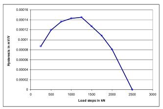
Figure7: Hysteresis behaviour for the transducer B-2.5kN
