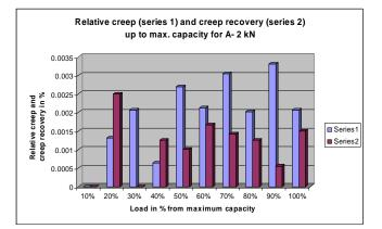
Figure 4: Relative creep and relative creep recovery in % versus load in % for A-2kN
