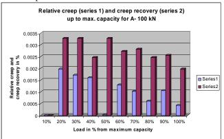
Figure 2: Relative creep and relative creep recovery in % versus Load in % for A-100kN
