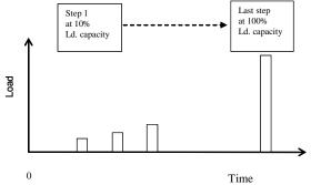
Figure 1: Scheme for loading each step from zero to max. Ld.
