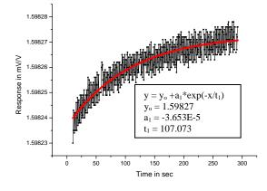
Figure 5: Creep behaviour for the transducer B-2.5kN at max. Ld.
