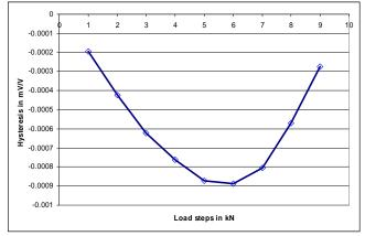
Figure8: Hysteresis behaviour for the transducer A-100kN
