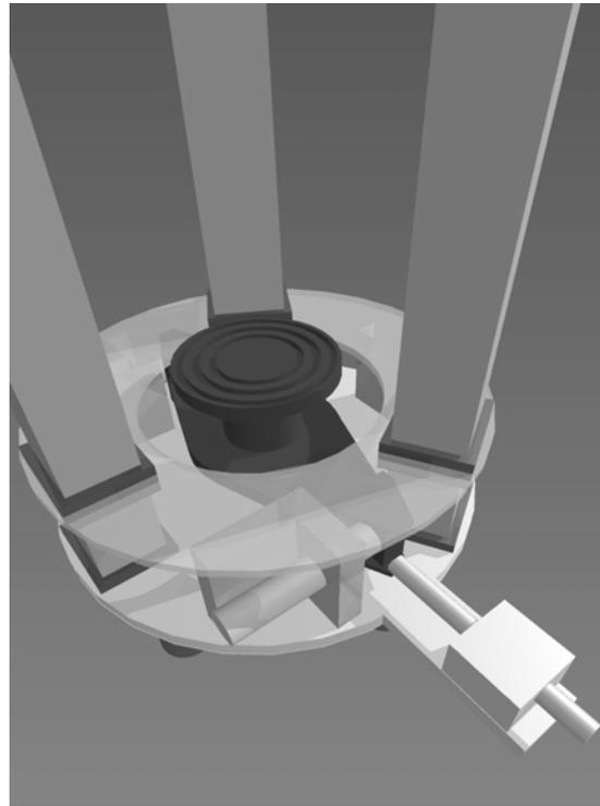
**Figure 2:** Base of the 1.1 MN·m TSM with actuating lever and electrical drives (computer design)
