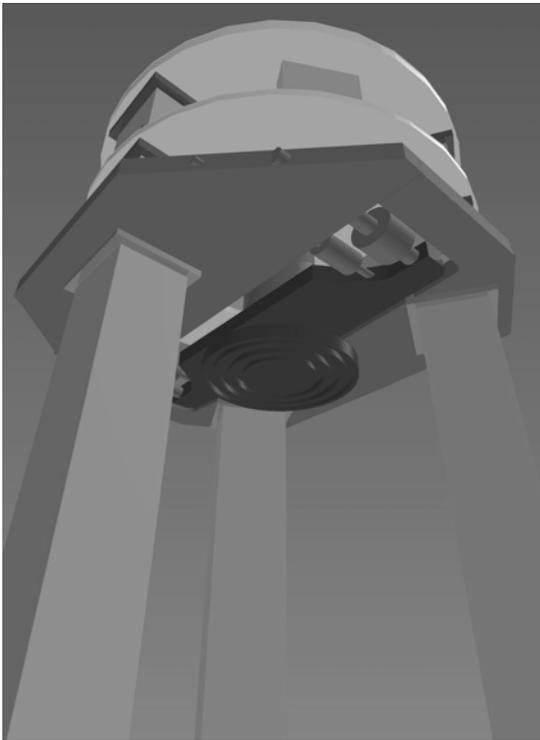
**Figure 1:** Top of the 1.1 MN·m TSM with force transducer sets acting on the measuring lever arm (computer design)
