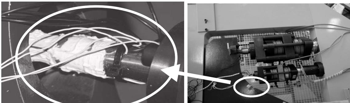
**Figure 3:** Force-transducer sets for 220 kN-m (small) and 1.1 MN-m (large) and elastic hinge element to measure the parasitic mechanical components in the contact area between force transducer and lever arm
