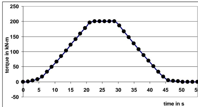
Figure 5: Typical loading diagram for 200 kN·m step
