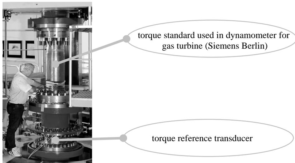
**Figure 4:** Device under test (700 kN·m) in line with the reference transducer (1.1 MN·m)
