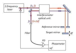
**Figure 3**: Agilent vibrometer system configuration.  $f_1$ ,  $f_2$  indicate the frequencies of the probe and reference beams, and *df* indicates the frequency shift due to the target mirror motion. PD: photodetector
