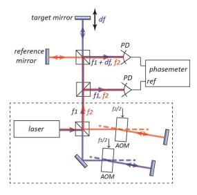
**Figure 4**: Custom auxiliary vibrometer configuration (simplified).  $f_1$ ,  $f_2$  indicate the frequencies of the probe and reference beams, and *df* indicates the frequency shift due to the target mirror motion. Dashed line encloses heterodyne-generation section. PD: photodetector; AOM: acousto-optic modulator.
