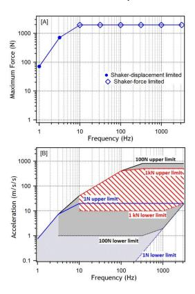
**Figure 5**: System operating limits. [A] shows the maximum force that can be applied to a transducer as a function of frequency. [B] shows the available range of acceleration values at each frequency, with limits achievable at different force levels indicated. In addition to the component specifications listed in Table 1, a minimum displacement criterion of 50 nm has been imposed, and a mass of 2 kg has been assumed for the transducer (with couplings).
