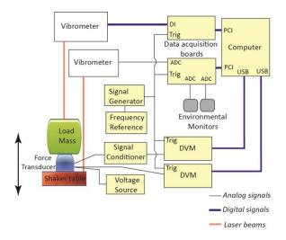
**Figure 2**. Calibration system configuration. Trig: trigger input, ADC: analog-to-digital converter, DI: digital input, PCI: PCI bus interface, USB: USB bus interface.
