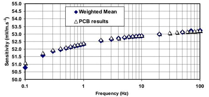
Figure 5. Weighted mean sensitivity for NPLI and TMS in comparison with the PCB sensitivity values in frequency range 0.1 Hz to 100 Hz.
