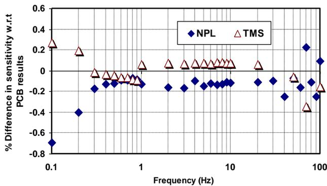
Figure 4. Relative difference of NPLI and TMS calibration results compared with PCB results
