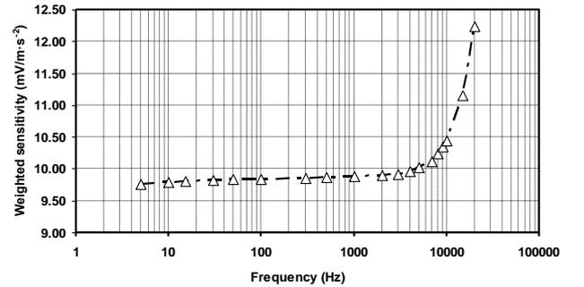
Figure 2. Weighted mean sensitivity for comparison in frequency range 5 Hz to 20 kHz for TMS and NPLI.
