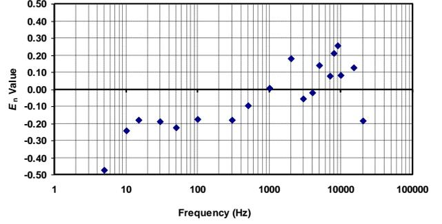
Figure 1.  $E_n$  values for the comparison in frequency range 5 Hz to 20 kHz between TMS and NPLI.
