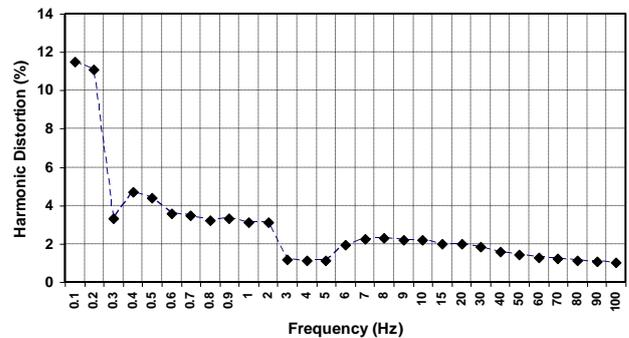
Figure 6. Harmonic distortion in low frequency measurements in range 0.1 Hz to 100 Hz.
