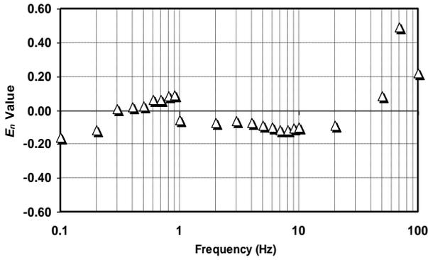
Figure 3.  $E_n$  value for the comparison in frequency range 0.1 Hz to 100 Hz between TMS and NPLI.
